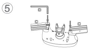
Use the Allen wrench  $\hfill \square$  and tighten the Allen screws from the bottom side of the spacer joints . This secures the spacer joints to the water shutoff valve.
