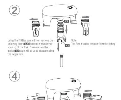
Align the grooves and slide the spacer joints (C) to
