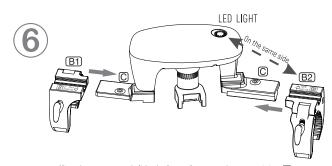
Align the grooves and slide the large clamps to the spacer joints . Note: Large clamp@2 should be attached on the side of the LED light. Both clamp knob handles should face towards the same direction.
