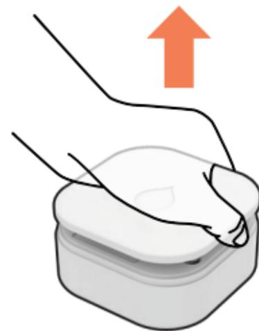
Remove the battery cover from the sensor.
