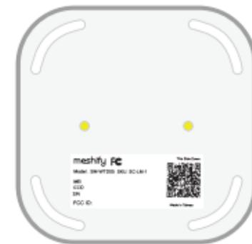
Place the sensor flat on the ground with the label facing down.
